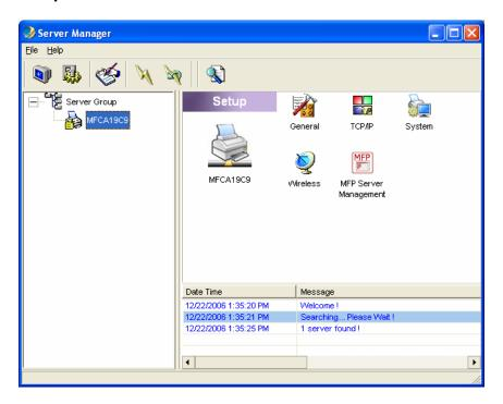
Click "Setup" icon on the tool bar, the setup items of the current selected MFP Server will be showed on the right side of the window.
